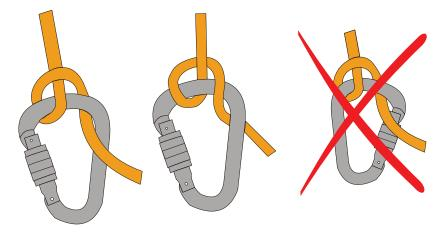
Used for lowering (of material, for self-rescue), can be used to belay the lead climber when using the climbing technique.
