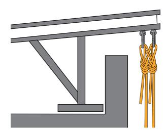
The bunny knot is suitable for anchoring to the points which are close to each other (< lm). In this case the advantage is tying only one knot which is easily adjusted to fit the required direction. The disadvantage is the need for longer rope if the anchor points are further apart.
