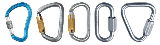
For work at heights we prefer using the connectors according to the EN 362 standard, which sets a minimum requirement of major axis strength 20 kN and at least two independent movements for opening (we recommend to use the connectors with screw lock or triple lock).
