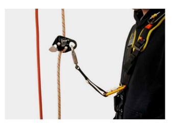
The function of the fall arrester is to arrest an unexpected fall caused by a failure of the work positioning system or an error of the user.
