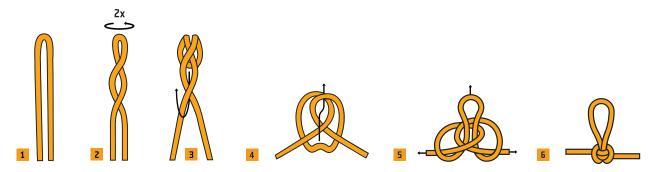
Used for anchoring in the middle of the rope, two-point anchoring (Y-hang), protecting the rope (bypass) by a steel sling, isolating a damaged part of the rope (it is a knot tied on the bight). Alpine butterfly reduces the strength of the rope by up to 39%
