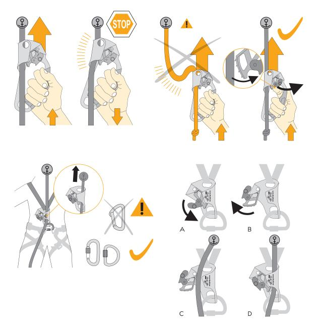
Used to reach the working position (ascent on rope). The main prerequisite for safe use is to prevent a fall on the ascender as there is a risk of damaging the rope and subsequent fall of the worker.
