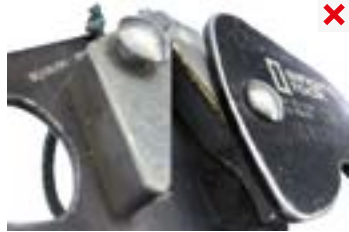
loss of material on sliding part of body
