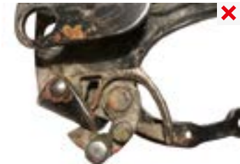
corroded - functionality limitation
