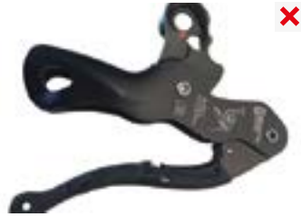
damaged regulation handle
