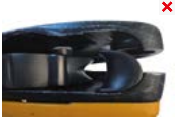
broken wire of the belay device
